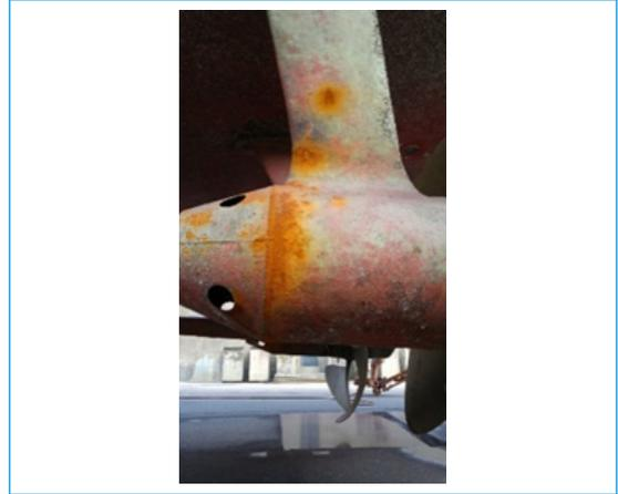
Figure 1. V-strut and barrel erosion
