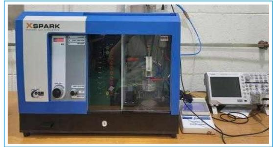
**Figure 1.** Electrostatic Discharge Sensitivity Tester
