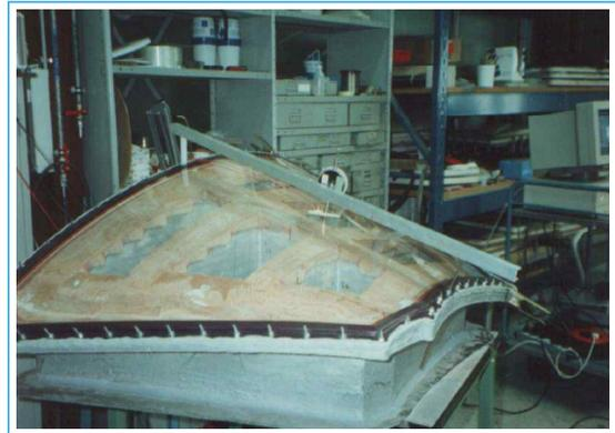
Figure 3. Prototype for windshield bird strike test
