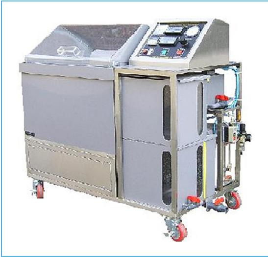
Figure 4. Configuration of test chamber for salt spray test
