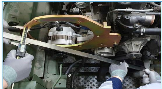
Figure 8. Measure the power transmission belt alignment
