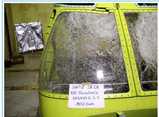
Figure 4. Result of windshield bird strike test
