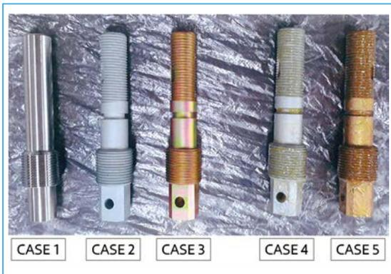
**Figure 3.** Configuration of simplified test specimens
