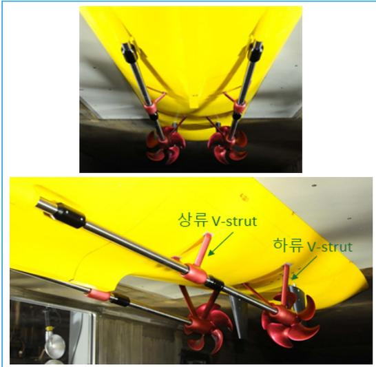
Figure 2. V-strut installed on the model ship
