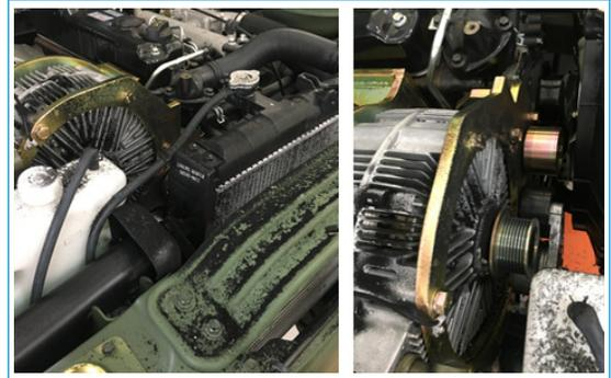
Figure 5. Belt break during the self-test
