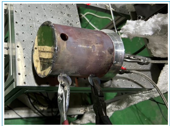
Figure 5. Burner for Radiation Experiment (close state)
